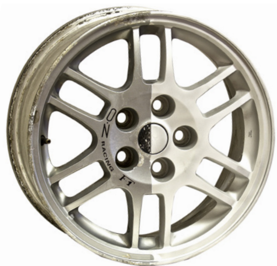
Alloy wheel before and after wet blasting
