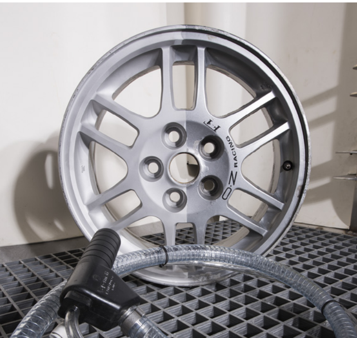
Alloy wheel after and before wet blasting in a Vapormatt Puma
